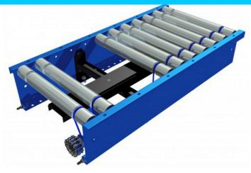
• A pneumatically operated rubber covered friction pad comes into contact with the underside of the rollers and gives negative line pressure over a standard brake length of 890mm.
