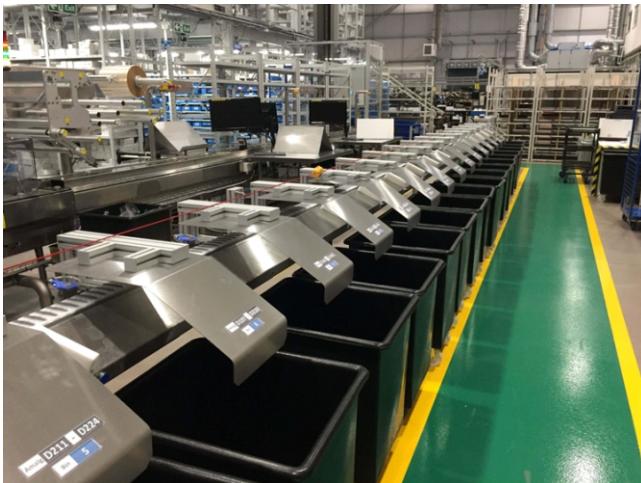
Sortation System for Flow Wrapped Packs using Air Nozzle Three Way Parcel Sortation with Barcode Scanning
