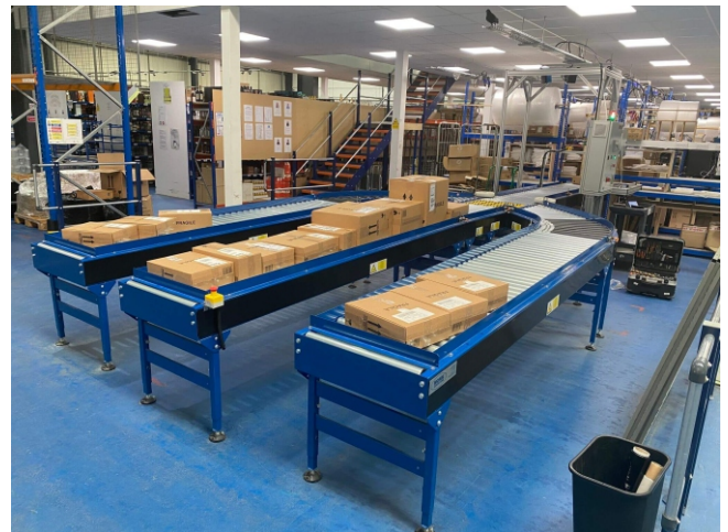
Sortation System for Flow Wrapped Packs using Air Nozzle Three Way Parcel Sortation with Barcode Scanning
