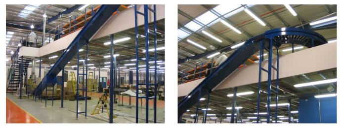
Tough PVC grip top or smooth belt material can be selected and floor to floor operation is guiet and smooth. A modular design means reduced installation time and low maintenance.
