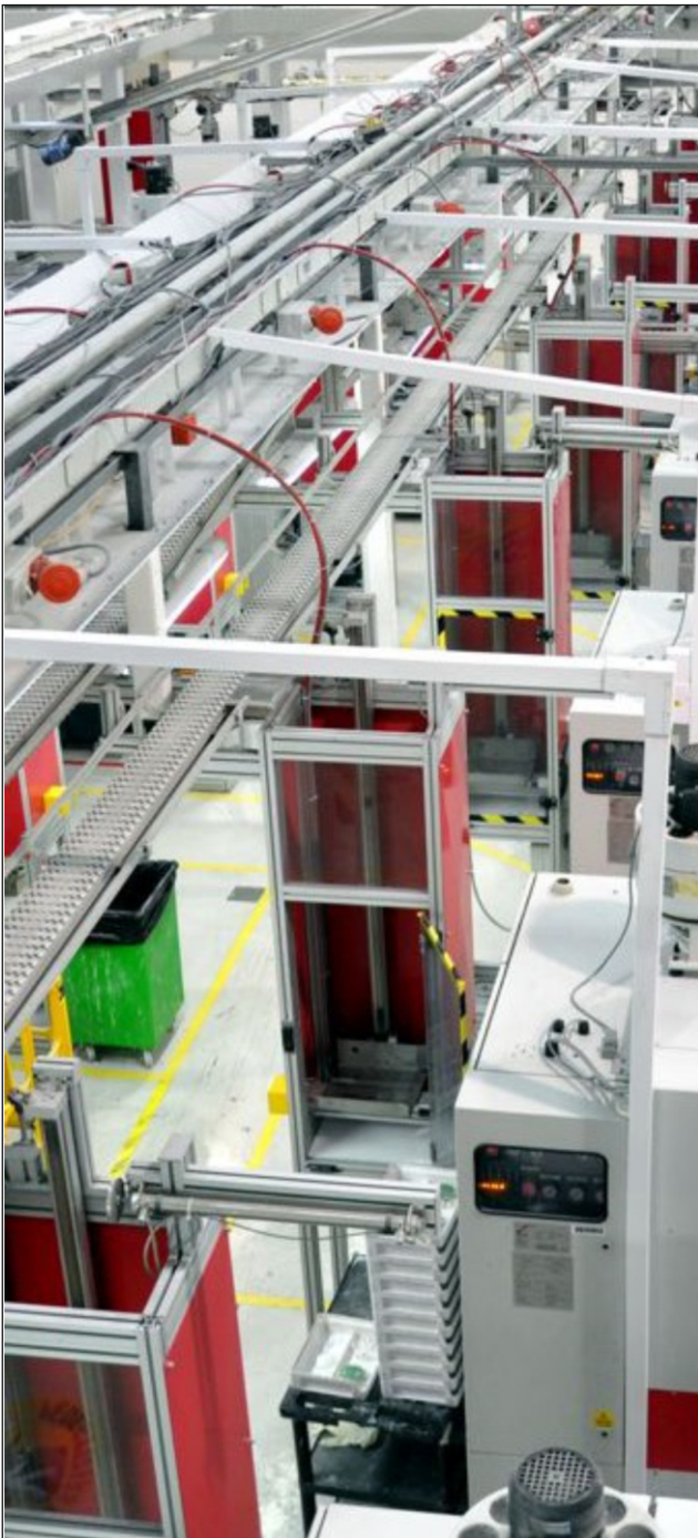
Row of automatic lifts used for transferring trays containing lenses from the lens producing machines up to the overhead conveyor system.
