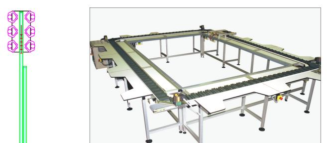
Constantly moving pallets with twin locations travel past nine operators as they assemble electronic components. The assemblies are then automatically transferred to the linear section of the line where the lids are loaded and then calibration and test are carried out.
