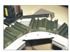
Corner modules allow pallets to turn through 90 degrees.
