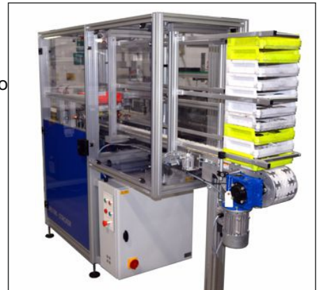
Stacking plastic trays at 20 trays per minute
