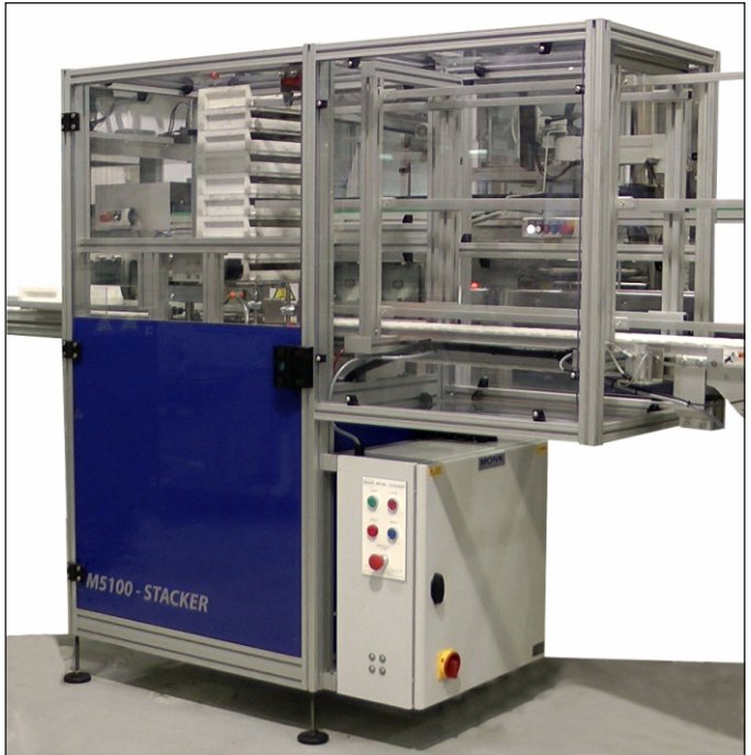
Stacking plastic trays at 20 trays per minute
