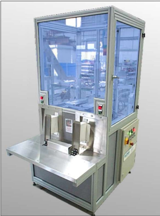
Carton filling machine viewed from the operator load and unload position.
