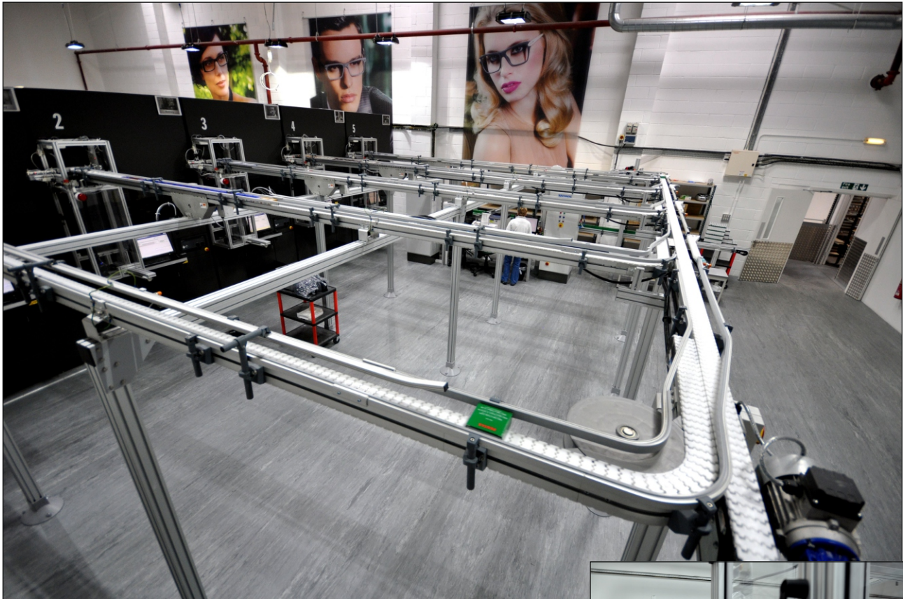
Infeed conveyors are installed at high level to allow good access
