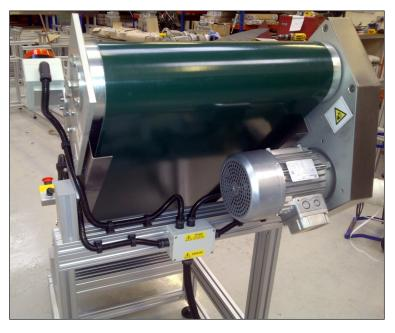
A special direct drive was designed with a toothed belt drive to the main drive roller.
