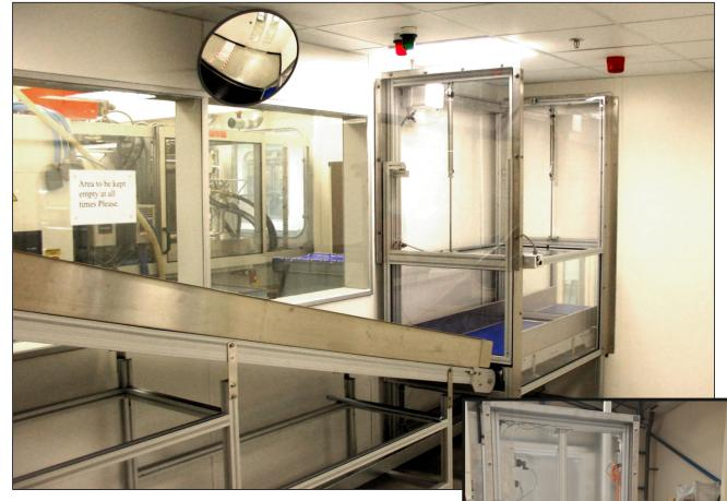
Our clean room air lock has integral conveyors, sealed vertical sliding doors.
