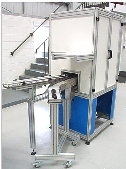
Vision Enclosures for automatically inspecting automotive brake pads ready for shipping to Federal Mogul.
