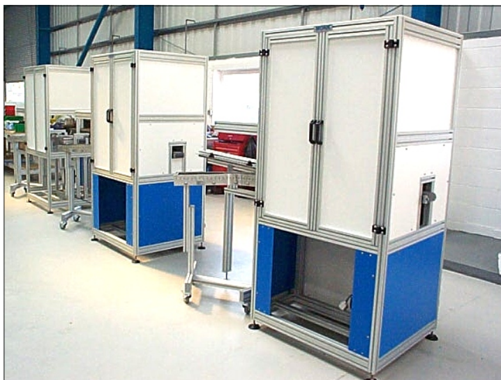
Vision Enclosures for automatically inspecting automotive brake pads ready for shipping to Federal Mogul.
