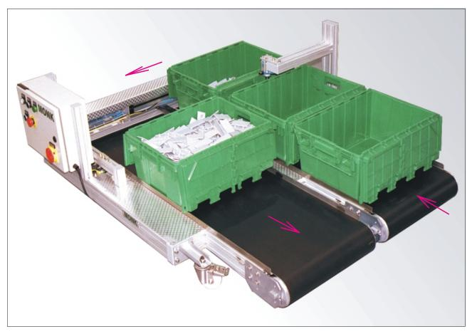
The **MONK BOX CHANGER** is a very efficient parts collection system allowing machines to operate unattended for long periods with parts storage boxes automatically queued and changed. They are used for the collection and storage of plastic mouldings, machined components etc..
