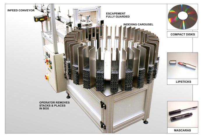
The **MONK AUTO-STACKER** saves labour when hand packing into boxes at the end of a production line. It automatically stacks product packs into a manageable stack sizes so that they will fit directly into a box.
