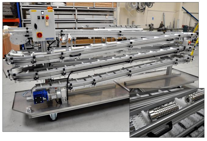
Our buffer storage system has been designed to store high precision machined components in separate compartments therefore eliminating damage.
