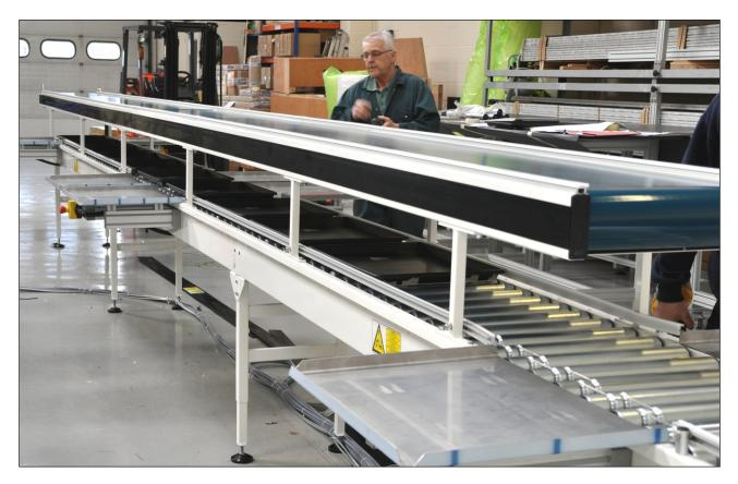
A 'Zero Line Pressure' roller conveyor and plastic trays are being used to collate items for a medical pack in a clean room before being sealed in plastic bags ready for dispatch.
