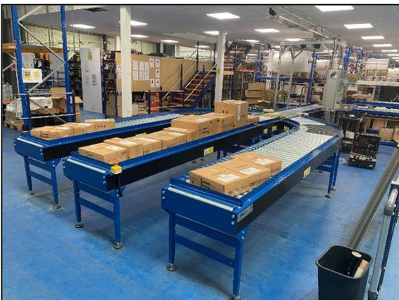
side belts, diverter arms, air blows and switch sorters as shown in this project. The switch sorter quickly diverts to one of three lanes without slowing the product down. Touch Screen displays make it easier for operators to run a system. Clear information is displayed and help screens can be added. Fault finding messages make it easier to find problems quickly.
