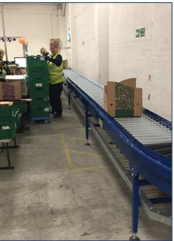
The system allows empty boxes to queue in front of operators. Boxes can then be packed and once complete they are released to the dispatch area. Each box is then controlled and released so operators can easily remove them from the line. Additional features were toggle switches for operators to be able to pause areas of the line, and variable speed controls.
