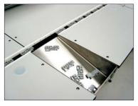
**AUTOMATIC EJECT**Automatic eject module with air jets to remove faulty assemblies.
