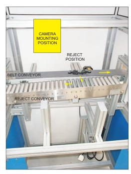
Inside the enclosure. Adjustable mountings for the camera, conveyor with rapid indexing up to a through beam sensor, reject position onto a roller conveyor.
