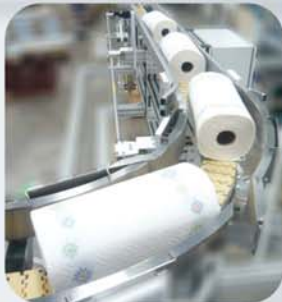
Conveyor with automated side guide
