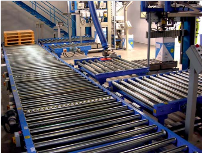
PALLET CONVEYORS. Heavy duty pallet roller conveyors for 800, 1000 & 1200mm wide pallets with loads up to 1500kg. 63mm diameter chain driven rollers. Supplied in standard lengths of 1588mm with individual drives for zero line pressure mode.
