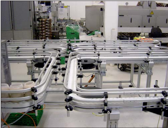
FLEX-CHAIN BUFFER STORE. Typical system handling Horlicks containers in the filling area. This system gives a 20 minute store by the side of the main production line.
