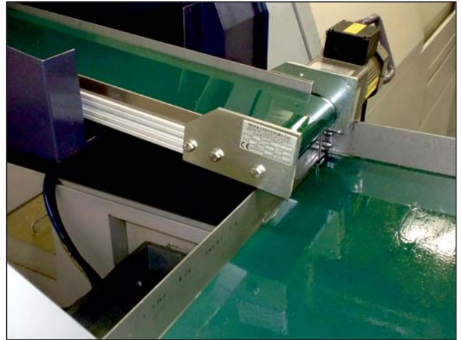
FLAT BELT CONVEYORS. Used here for unloading finished components from a machining center. Drip trays are used to collect the cutting oil and return it to the system.
