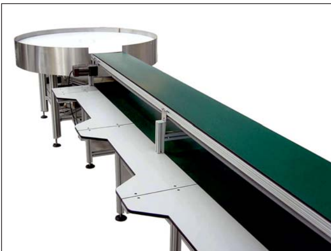
ROTATING STORAGE TABLES. Used for creating a buffer store at the end of a line, products are fed onto the table as it slowly rotates. An operator will then visit the table and pack or transfer the product back into the line.
