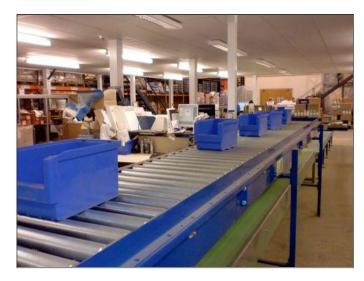
Operatives could then remove a tote for packing and the system would drive remaining totes forward. Therefore they would always have a continual flow of work.
