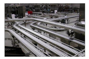
The outfeed system handled 605mm x 400mm x 150mm plastic baskets fed on a two tier stainless steel roller conveyor system. Empty baskets feed in on the lower level and once filled, full baskets would merge onto one outfeed line.
