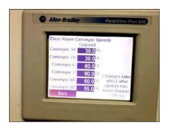
An HMI touch screen allows operators to make adjustments to the running speed of the line and give useful running information
