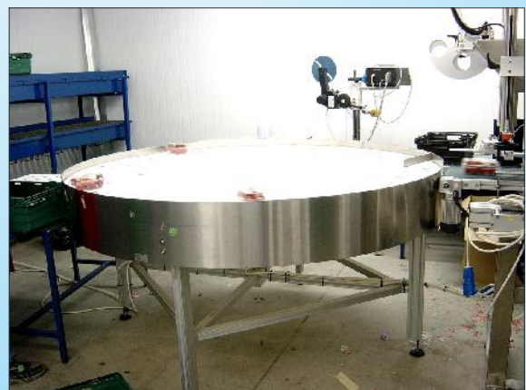
Rotating storage table 'C' where punnets collect, ready for immediate delivery to the super markets.
