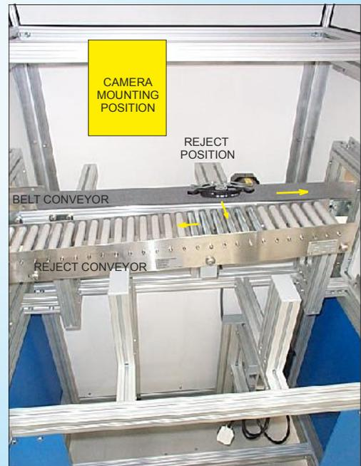
Inside the enclosure. Adjustable mountings for the camera, conveyor with rapid indexing up to a through beam sensor, reject position onto a roller conveyor.
