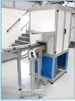
Rejects are automatically returned to the operator on a gravity roller conveyor for re-working.
