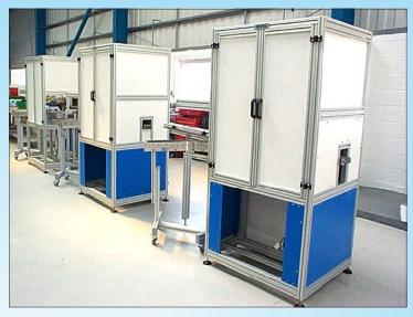
Vision Enclosures for automatically inspecting automotive brake pads ready for shipping to Federal Mogul.
