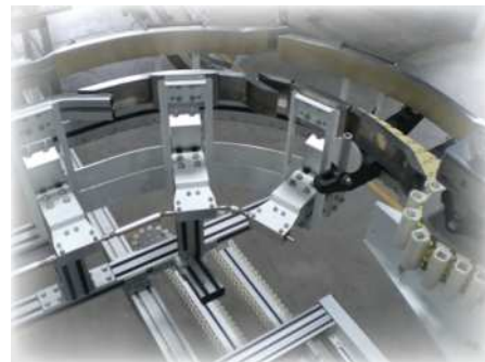
Automated side guide installed at bend section
