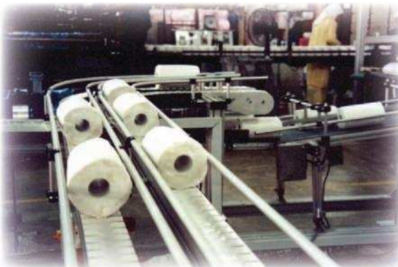
Vertical diverter & conveyor system for kitchen towel
